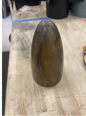
Figure 16: Molded subscale elliptical nose cone
