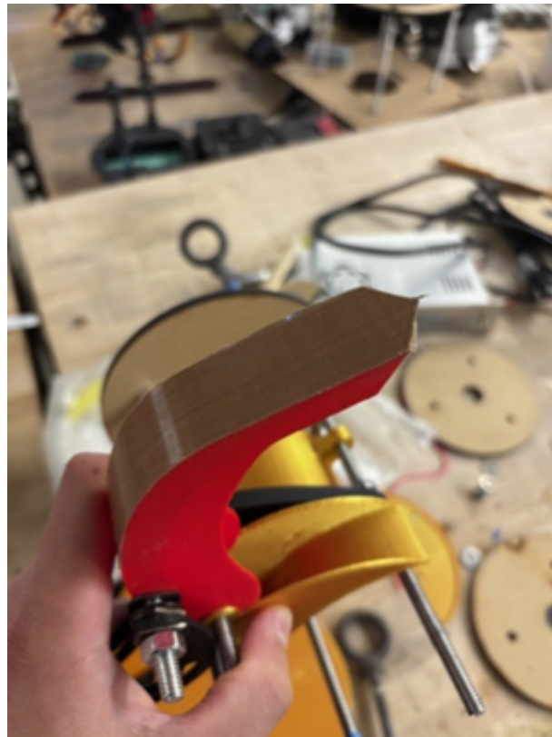
Figure 75: Current shovel design including PTFE on back and one tooth to decrease failure points.
