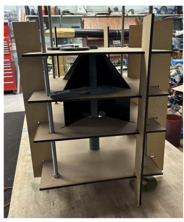
Figure 39: Subscale Tail Section Fabrication Jig
